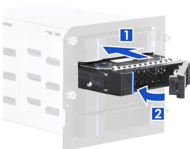
Figure 22 3.5" hot-swap HDD tray installation
