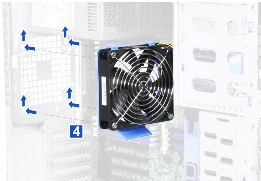
Figure 29 Rear fan maintenance step-2
