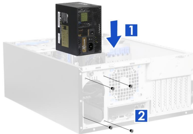
Figure 30 Single PSU installation
